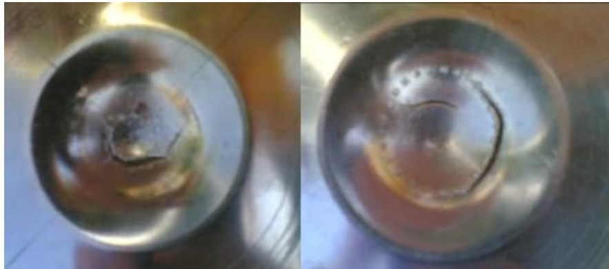
Figure (11): Models containing defects of large size.
